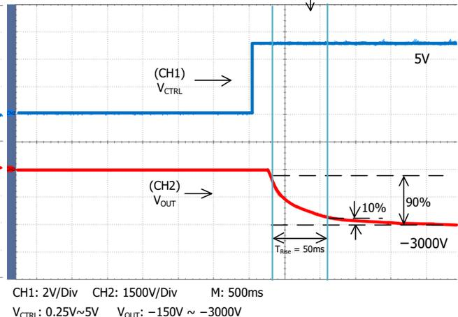
Figure 12. Rising Trail for Large Signal Response
