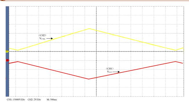
$V_{CTRL} \colon 0.25 V \sim 5 V \qquad V_{OUT} \colon \text{-}1400 V \sim \text{-}30000 V$
