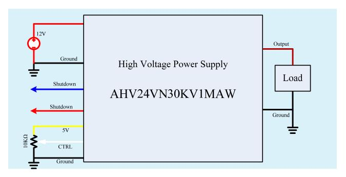
Figure 8. Controlled by Potentiometer
