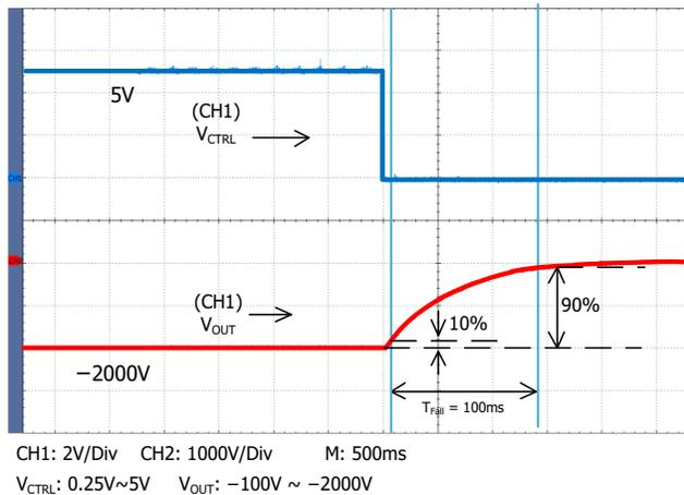
Figure 11. Falling Trail for Large Signal Response
