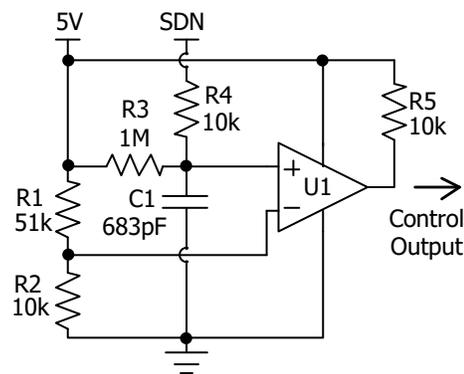
Figure 6. The Equivalent Circuit for SDN Port
