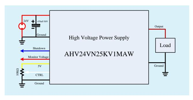
Figure 8. Figure 8. Control by External Signal Source
