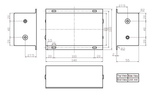
Figure 11. Dimensions for AHV24VN25KV1MAW
