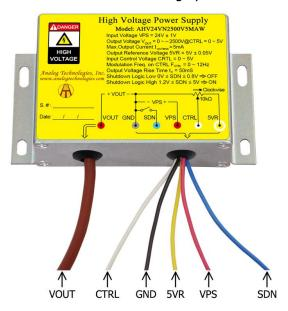
Figure 2. The Connecting Lead Wires of AHV24VN2500V5MAW
