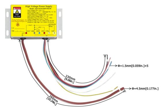
Figure 13. Connecting Lead Wires of AHV24VN2500V5MAW
