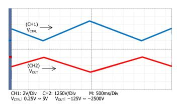
Figure 8. Triangle Wave Modulation
