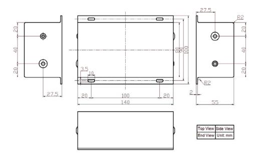
Figure 11. Dimensions for AHV24VN15KV1MAW
