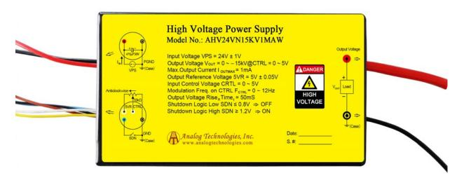
Figure 1. Physical Photo of AHV24VN15KV1MAW
