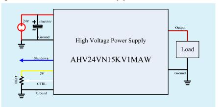
Figure 8. Control by External Signal Source
