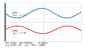
Figure 9. Sine Wave Modulation
