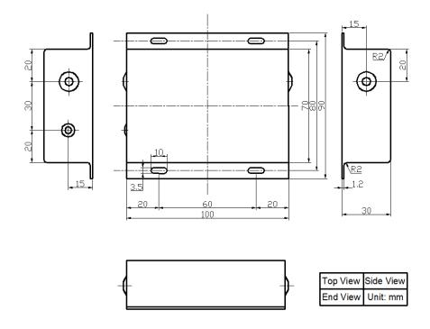
Figure 11. Dimensions for AHV24VN10KV2MAW
