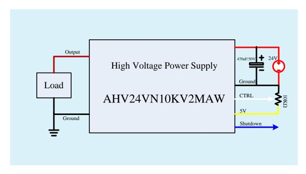
Figure 8. Control by External Signal Source
