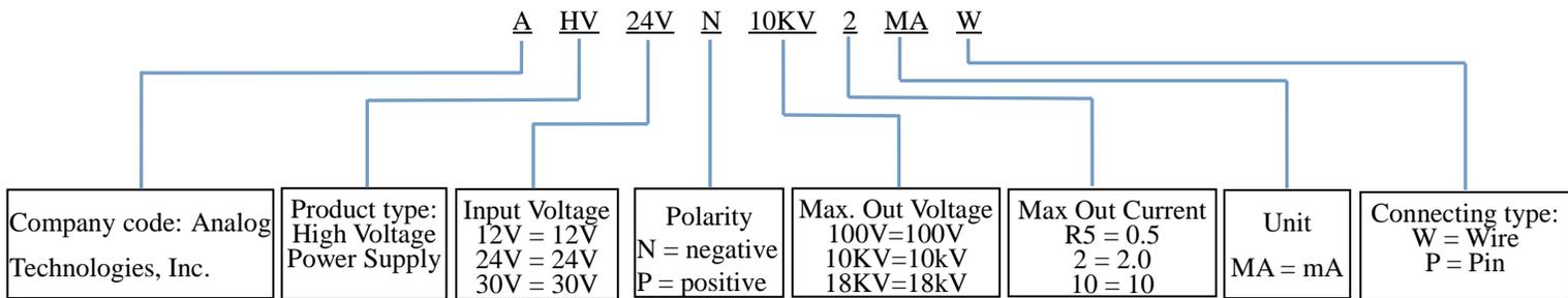
Figure 9. Naming Rules of AHV24V10KV2MAW
