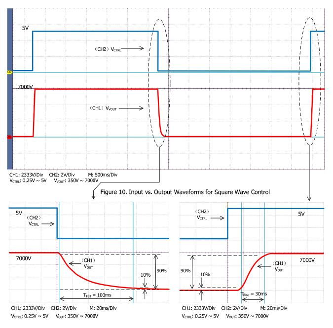
Figure 11. Falling Trail for Large Signal Response
