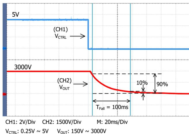
Figure 11. Falling Trail for Large Signal Response
