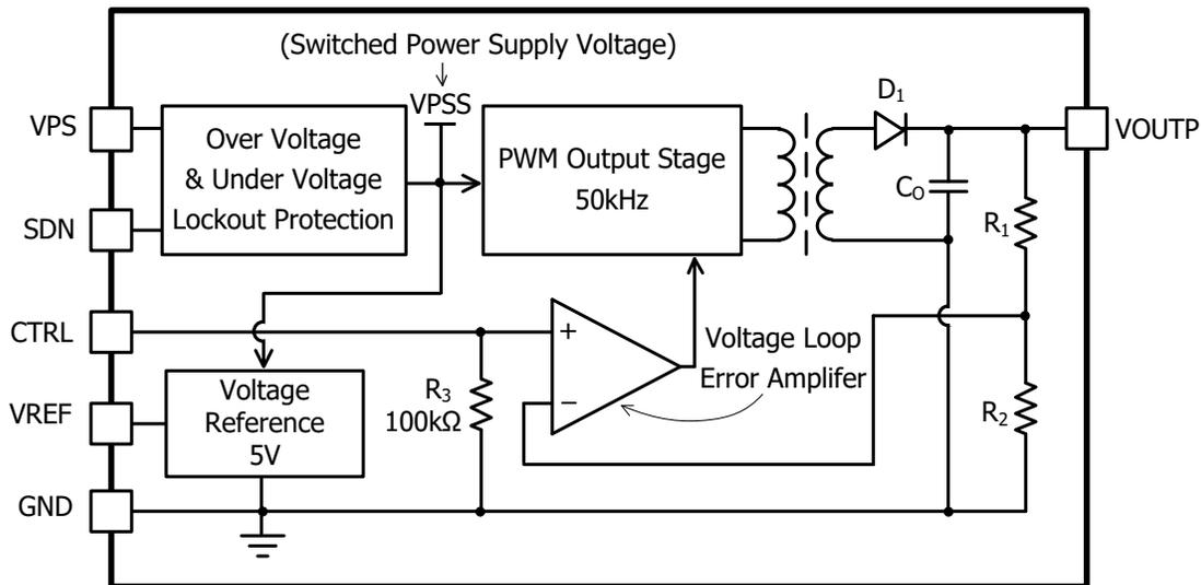
$V_{OUTP} = N \times V_{CTRL}$ , where  $N$  is the amplification factor:  $N = R_1/R_2$ .
