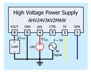
Figure 4. Modulating Output by an AC Signal Source
