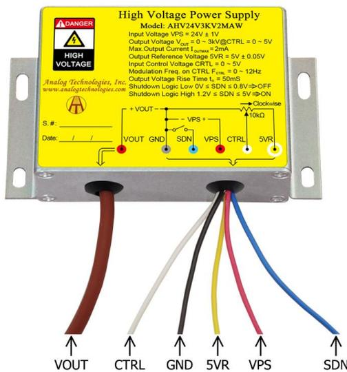
Figure 2. The Connecting Lead Wires of AHV24V3KV2MAW
