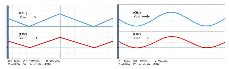
Figure 8. Triangle Wave Modulation
