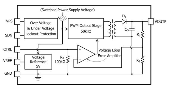
VOUTP =  $N \times V_{CTRL}$ , where N is the amplification factor:  $N = R_1/R_2$ .
