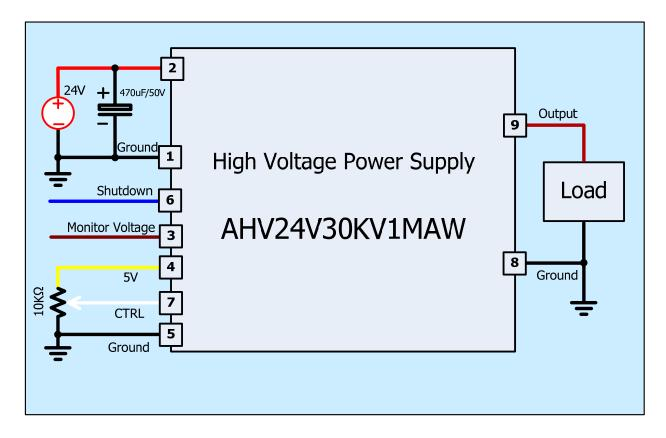
Figure 3. Setting Output to be a Constant Voltage
