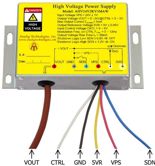
Figure 2. The Connecting Lead Wires of AHV24V2KV3MAW
