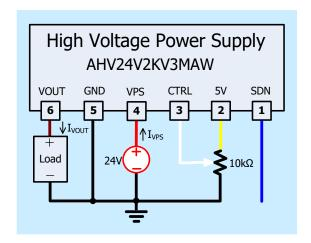
Figure 3. Setting Output to be a Constant Voltage
