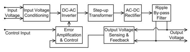
Figure 10. Block Diagram
