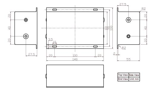
Figure 12. Dimensions for AHV24V25KV1MAW
