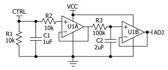
Figure 5. The Equivalent Circuit for CTRL Port
