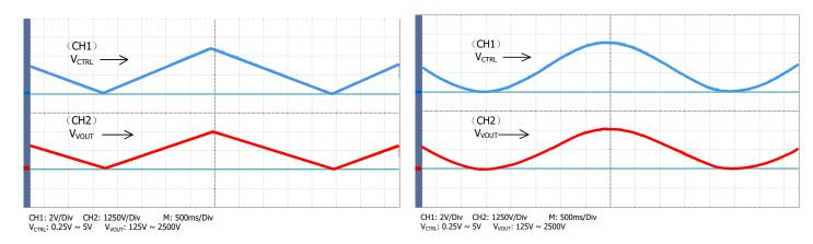
Figure 8. Triangle Wave Modulation
