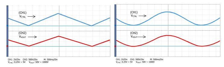
Figure 8. Triangle Wave Modulation
