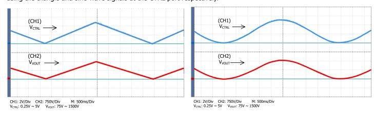
Figure 8. Triangle Wave Modulation
