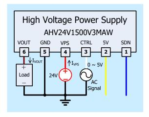
Figure 4. Modulating Output by an AC Signal Source
