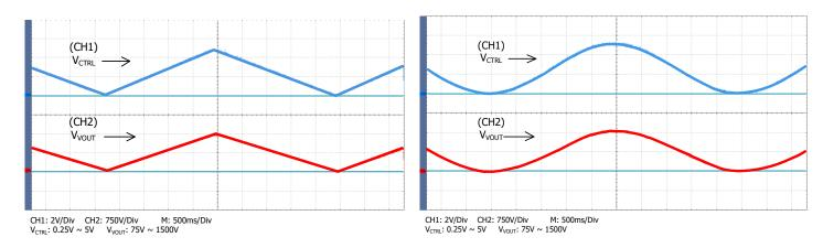
Figure 8. Triangle Wave Modulation
