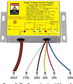
Figure 2. The Connecting Lead Wires of AHV24V1500V10MAW
