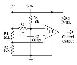
Figure 6. The Equivalent Circuit for SDN Port
