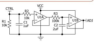
Figure 5. The Equivalent Circuit for CTRL Port
