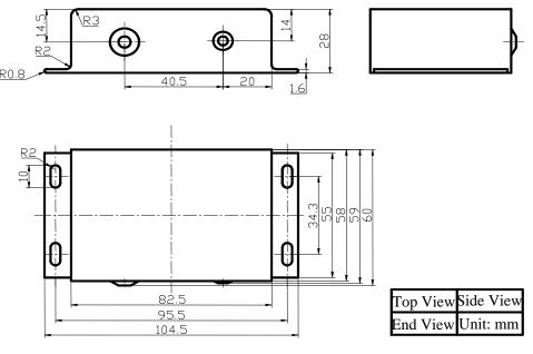
Figure 12. Dimensions for AHV24V10KVR6MAW
