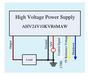
Figure 8. Control by External Signal Source
