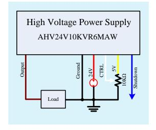
Figure 9. Constant Output Voltage
