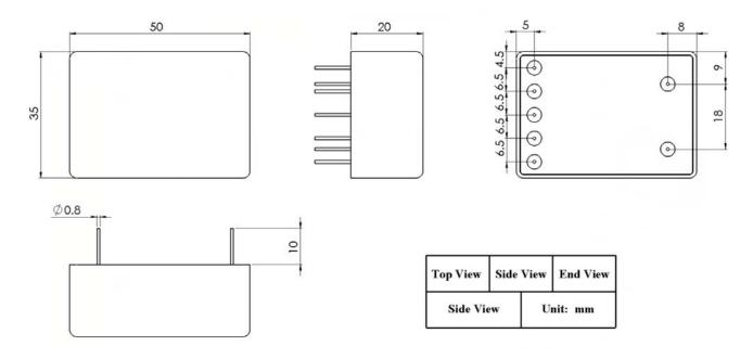
Figure 13. Dimensions for AHV12V2KVR5MAP
