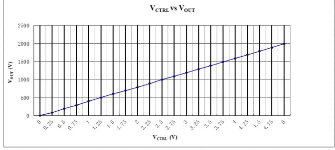
High voltage power supply testing data (Test condition: the load is 4  $\mbox{M}\Omega)$
