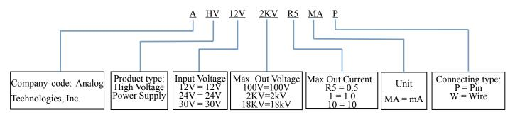
Figure 10. Naming Principle of AHV12V2KVR5MAP
