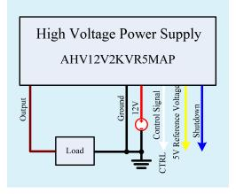
Figure 8. Control by External Signal Source
