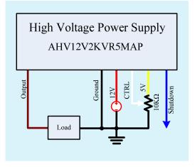
Figure 9. Constant Output Voltage
