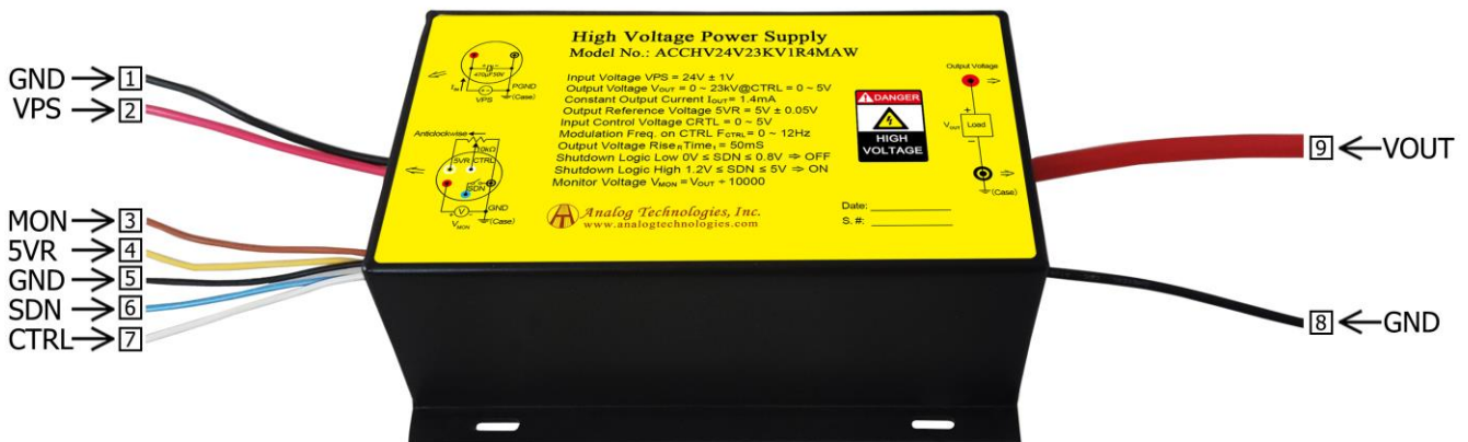
Figure 2. The Connecting Lead Wires of ACCHV24V23KV1R4MAW
