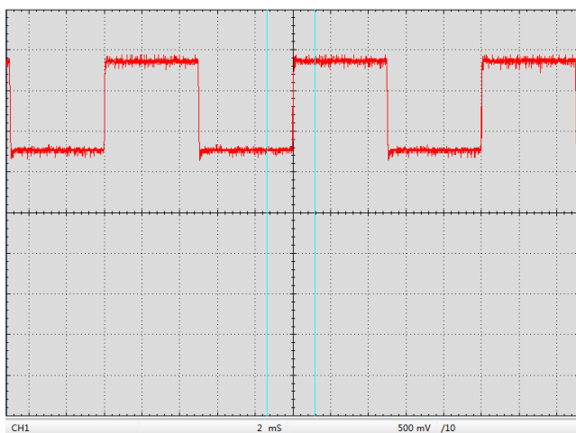
Figure 6. Digital Modulation Response at LDA Pin
