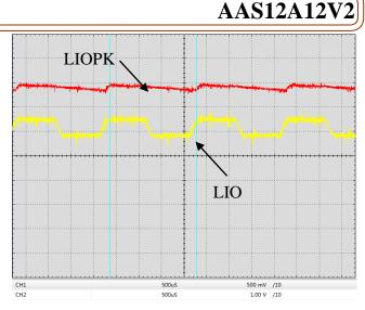
Figure 13. Digital Modulation Response at LIOPK & LIO Pin (f=500Hz)
