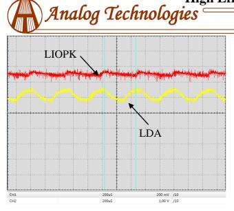
Figure 16. Digital Modulation Response at LIOPK & LDA Pin (f=2kHz)
