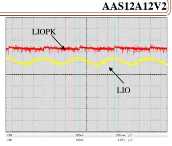
Figure 19. Digital Modulation Response at LIOPK & LIO Pin (f=3kHz)
