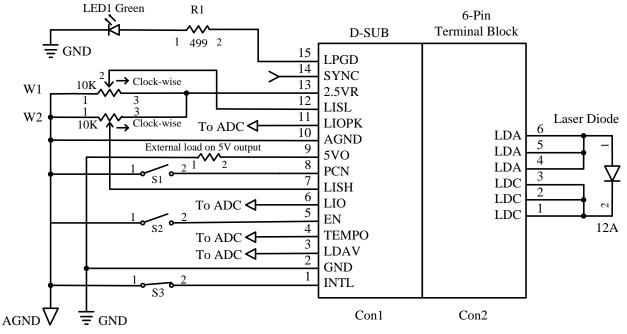
Figure 4. A Typical Application Schematic
