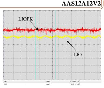
Figure 25. Digital Modulation Response at LIOPK & LIO Pin (f=6kHz)
