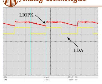
Figure 10. Digital Modulation Response at LIOPK & LDA Pin (f=100Hz)
