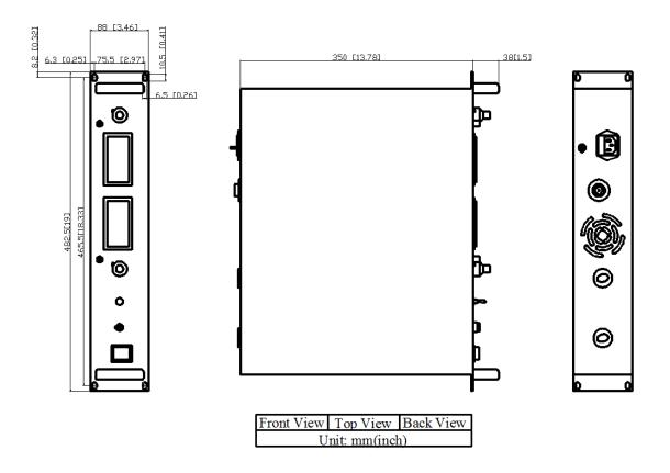
Figure 9. Dimensions for A2UHVAC3KV50MAIRM
