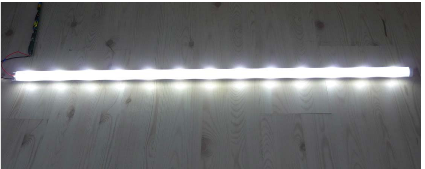
Figure 3. Full View of Light High Efficiency T8 LED Tube
