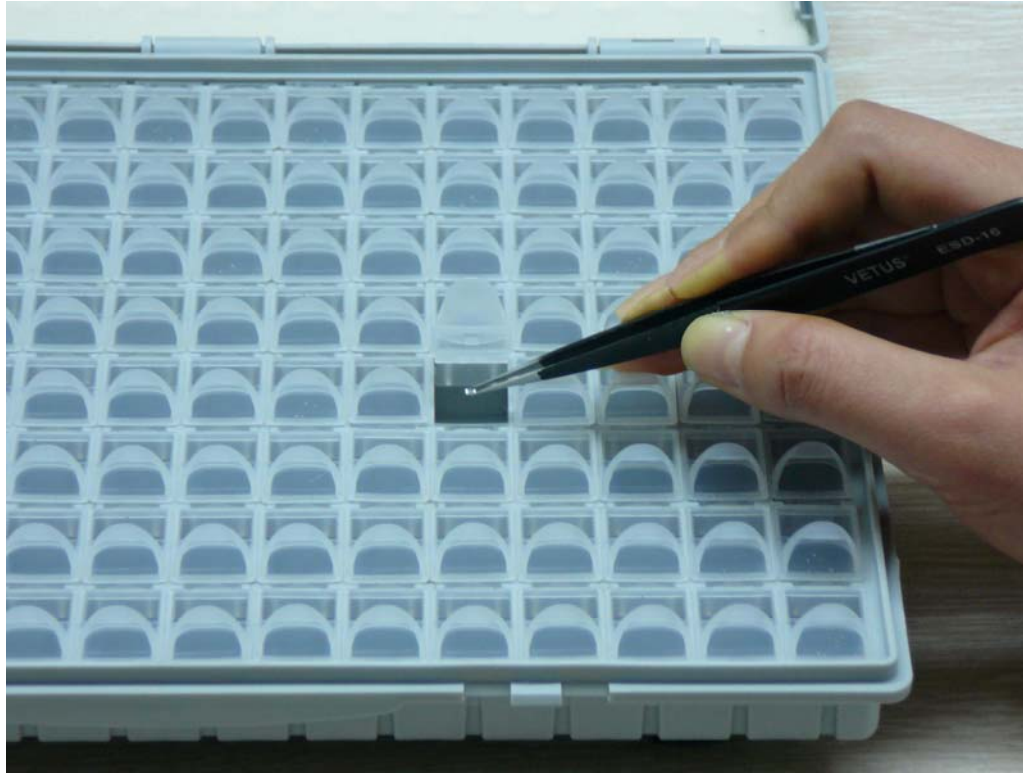
Figure 12. Storing or Obtaining an SMT Component
