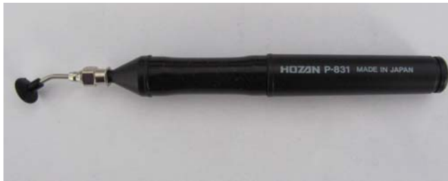
Figure 2. The Photo of Actual Vacuum Pen
