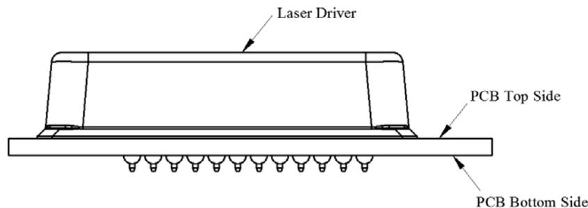
Figure 20. End View of the PCB Foot-print
