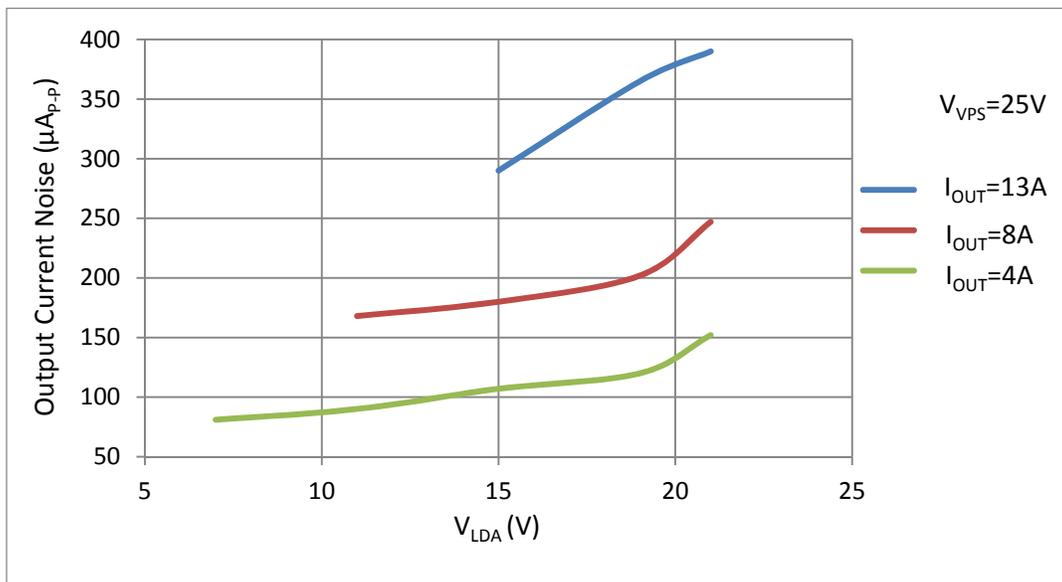
Figure 10.  $V_{\text{LDA}}$  vs. Output Current Noise@0.1Hz~10Hz
