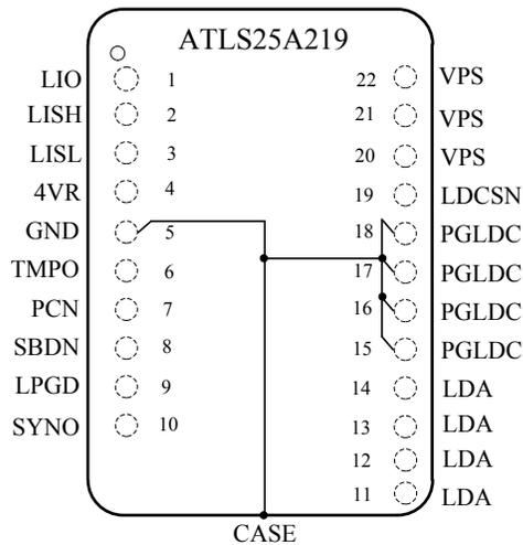
Figure 2 is the top view of the ATLS25A219D, which also shows the pin names and locations. Its thickness is 4.5mm. The pin functions and specifications are described in Table 1 below. Note that the metal case is internally connected to ground.
