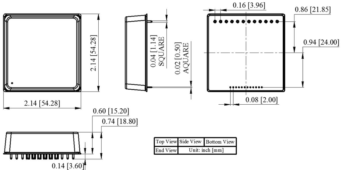
Figure 19. Dimensions of the DIP Package Driver
