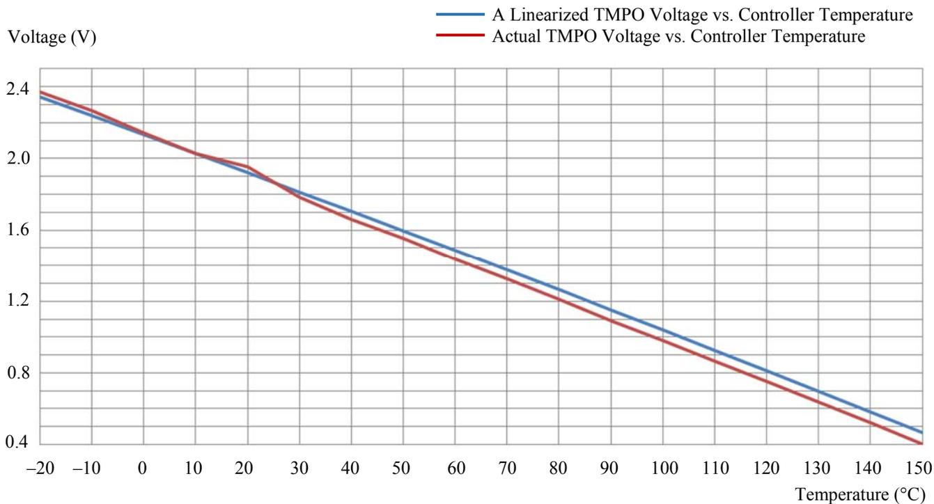
Figure 5. Controller Internal Temperature vs. TMPO Voltage
