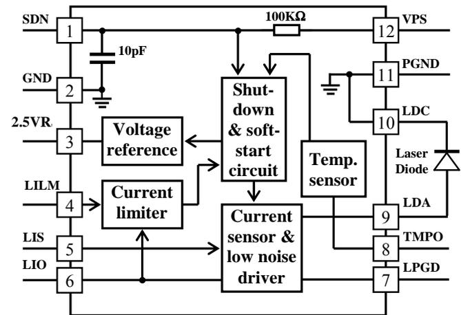
Figure 3. Block Diagram
