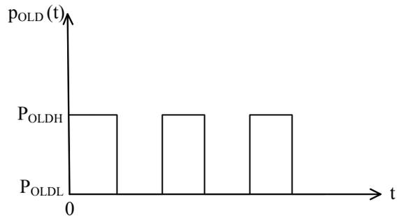
Figure 13. Laser Diode Optical Power p\_OLD Waveform
