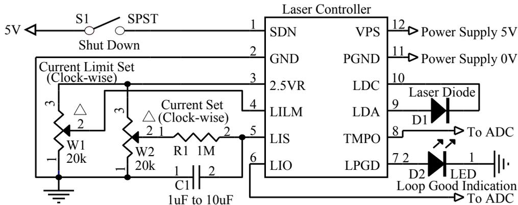
Figure 4.2. Typical Stand-alone Application Schematic for ATLS250MA103-PD
