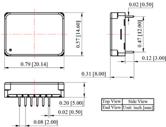
Figure 19. Dimensions of the DIP Package Controller
