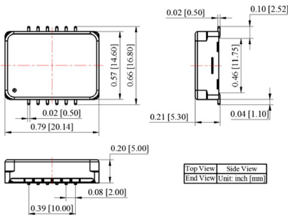
Figure 20. Dimensions of the SMT Package Controller
