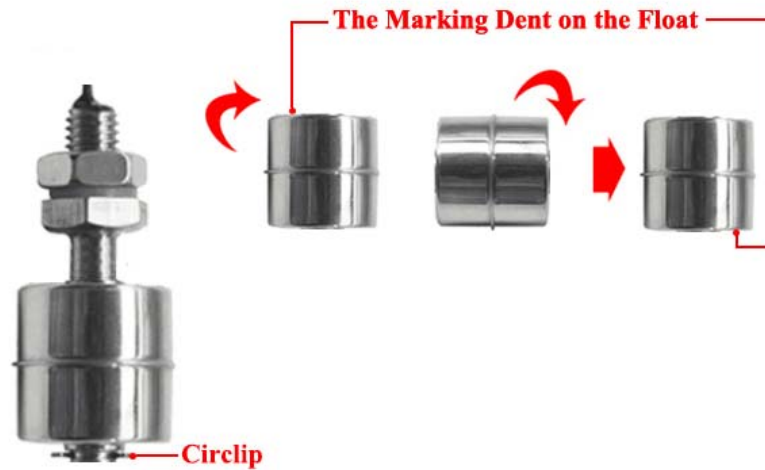
Figure 5. Swapping Float Orientation for Normally Open or Normally Closed
