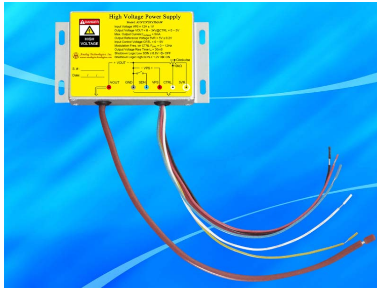
Figure 11. Leads of AHV12V3KV5MAW
