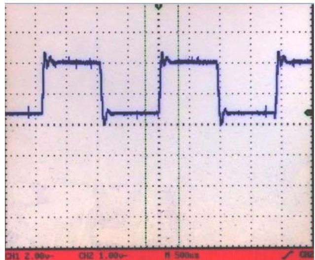
Figure 6. Digital Modulation Response at LDA Pin
