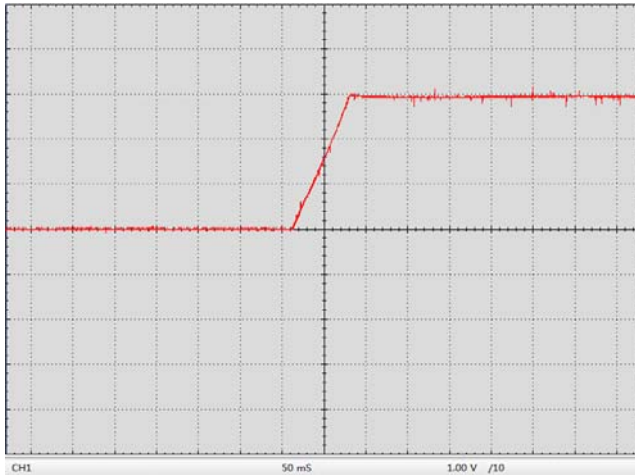
Figure 26. Start-up Waveform at LDA Pin
