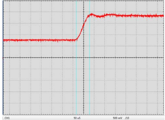
Figure 7. Digital Modulation Response at LDA Pin
