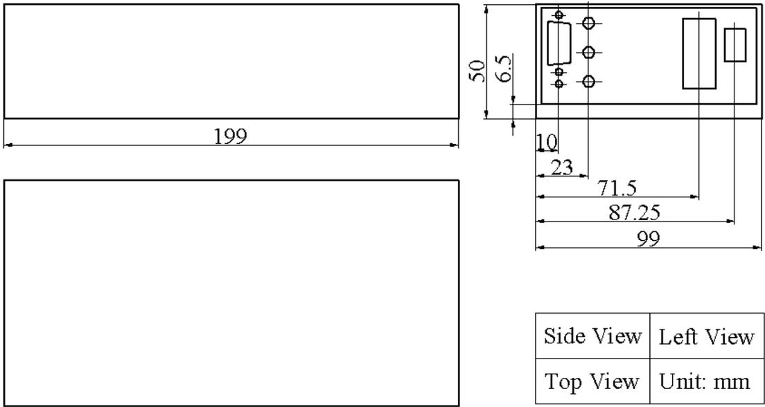
Figure 9. Mechanical Dimensions
