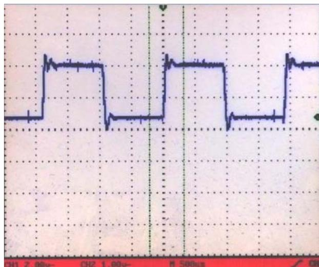
**Figure 6. Digital Modulation Response at LDA Pin**
