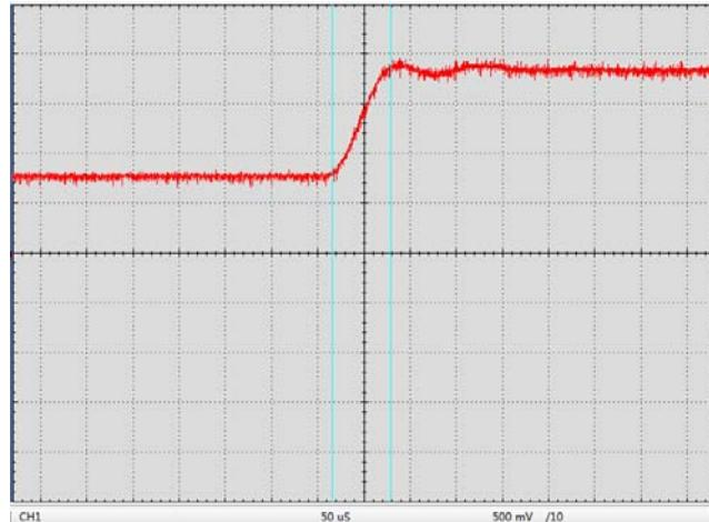
Figure 5. Digital Modulation Response at LDA Pin
