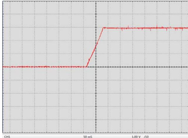
Figure 15. Start-up Waveform at LDA Pin
