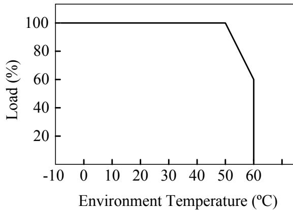
Figure 14. Derating Curve
