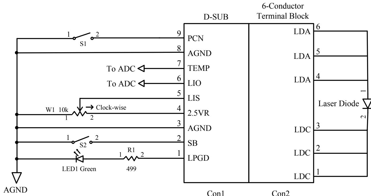
Figure 2. A Typical Application Schematic
