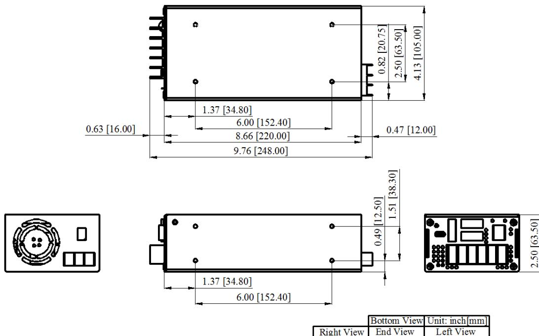
Figure 17. Mechanical Dimensions
