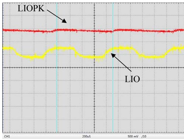
Figure 13. Digital Modulation Response at LIOPK & LIO Pin (f = 1kHz)
