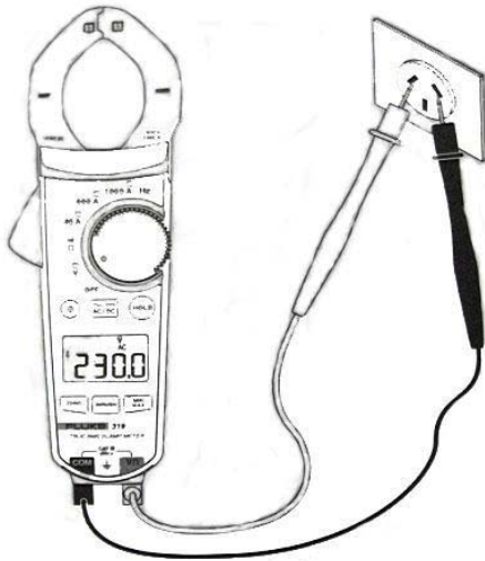
Figure 6. AC Voltage Measurement
